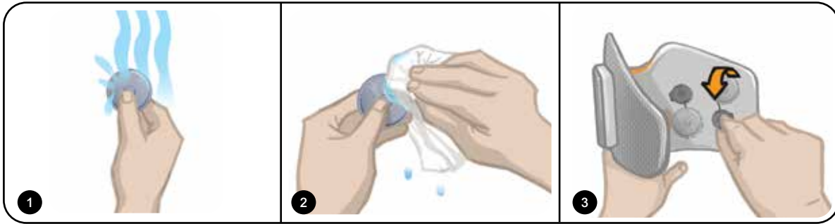
Figure 8-11: Fitting the Round Cloth Electrode
