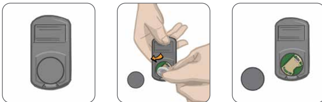
Figure 11-2: Replacing the Control Unit Battery
