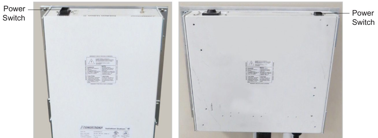
Figure 4-1: Location of Power Switch on the two models of Power Supply Boxes
