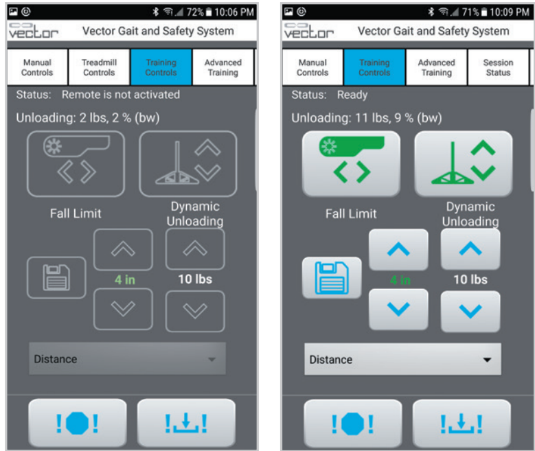
Figure 9-6: Example of Status Displays for Remote Control (Left) Remote Is Not In Control of Trolley, (Right) Remote Is In Control of Trolley
