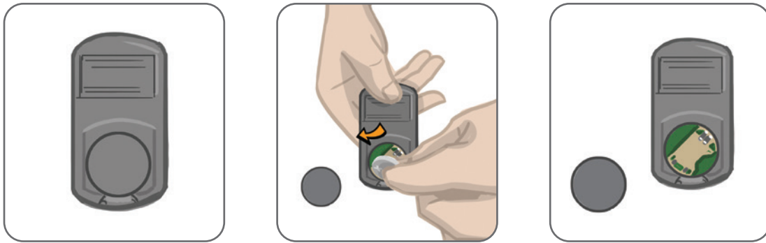
Figure 11-6: Replacing the Control Unit Battery
